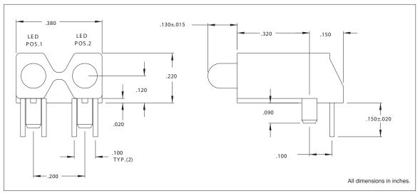
•2 T-1 LEDs mounted in single block. •Height and spacing alignment saves assembly cost.
