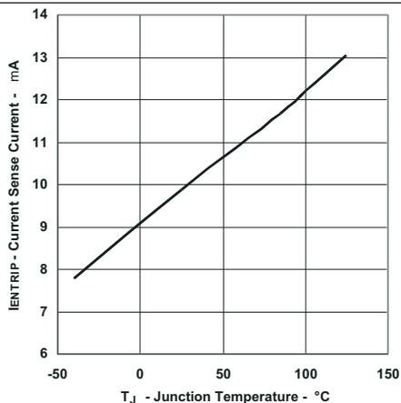
Figure 9. Current Sense Current vs Junction Temperature
