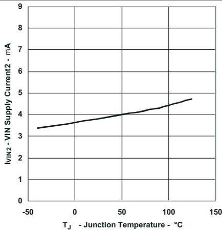
Figure 3. VIN Supply Current2 vs Junction Temperature
