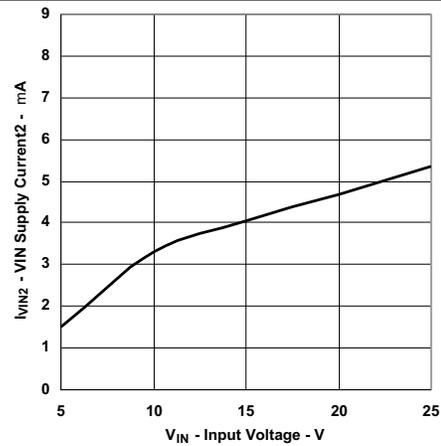
Figure 4. VIN Supply Current2 vs Input Voltage
