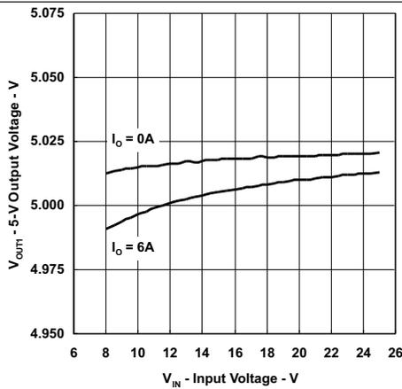
Figure 25. 5-V Output Voltage vs Input Voltage
