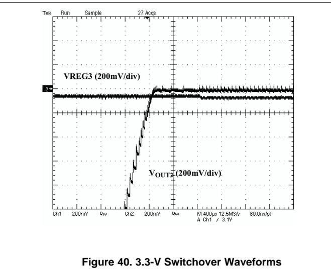
Figure 40. 3.3-V Switchover Waveforms
