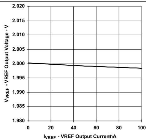
Figure 22. VREF Output Voltage vs Output Current
