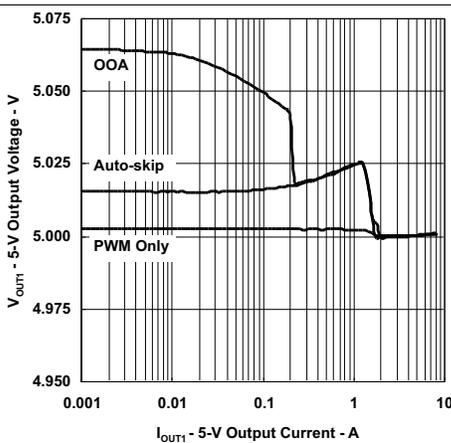
Figure 23. 5-V Output Voltage vs Output Current
