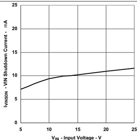
Figure 8. VIN Shutdown Current vs Input Voltage
