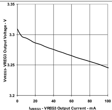
Figure 21. VREG3 Output Voltage vs Output Current
