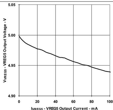
Figure 20. VREG5 Output Voltage vs Output Current
