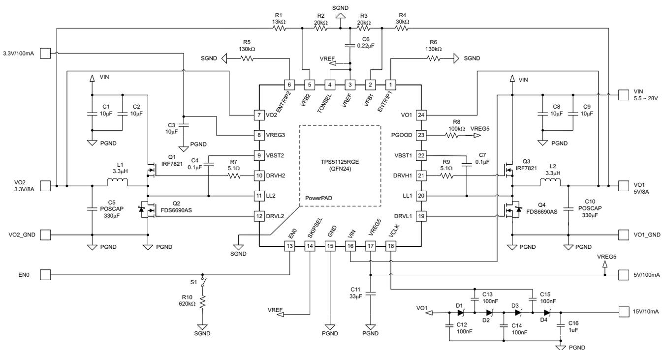
Figure 34. 5-V/8-A, 3.3-V/8-A Application Circuit (245-kHz/305-kHz Setting)
