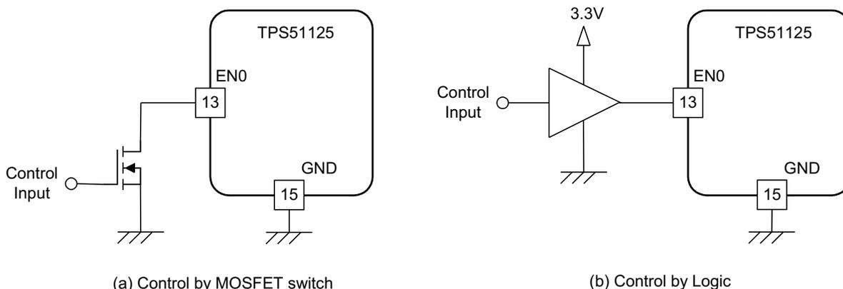
Figure 32. Control Example of EN0 Master Enable
