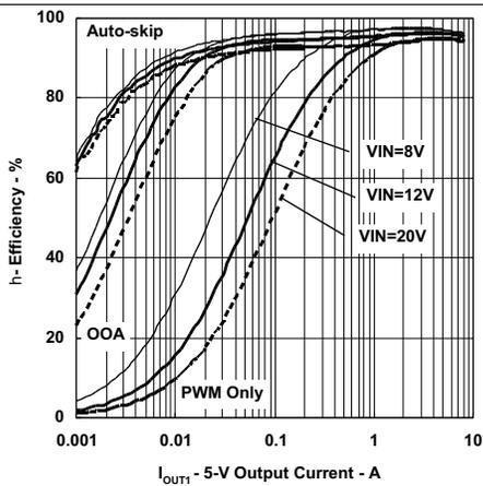
Figure 27. 5-V Efficiency vs Output Current
