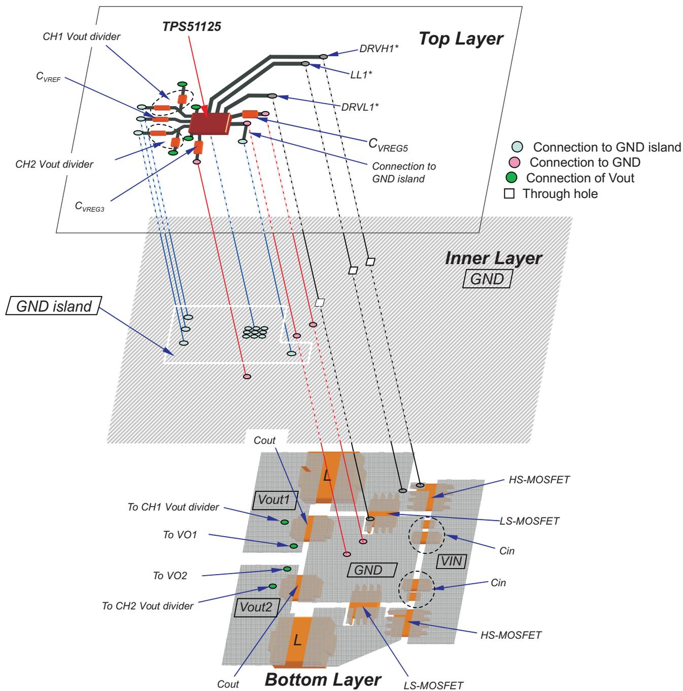
Figure 44. PCB Layout
