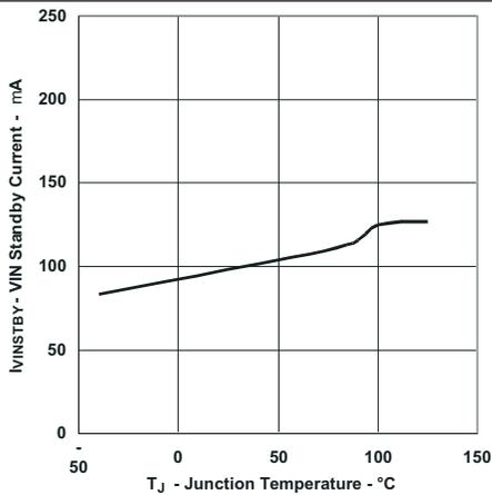
Figure 5. VIN Standby Current vs Junction Temperature
