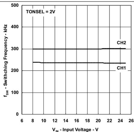
Figure 12. Switching Frequency vs Input Voltage
