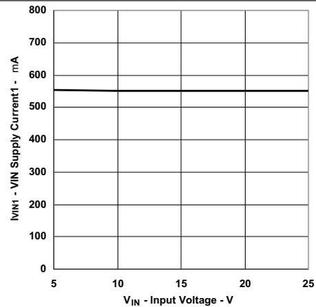
Figure 2. VIN Supply Current1 vs Input Voltage
