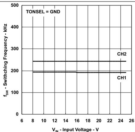
Figure 11. Switching Frequency vs Input Voltage
