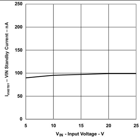
Figure 6. VIN Standby Current vs Input Voltage
