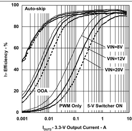
Figure 28. 3.3-V Efficiency vs Output Current
