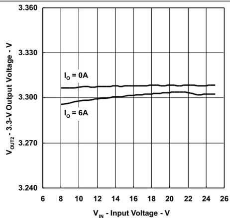
Figure 26. 3.3-V Output Voltage vs Input Voltage
