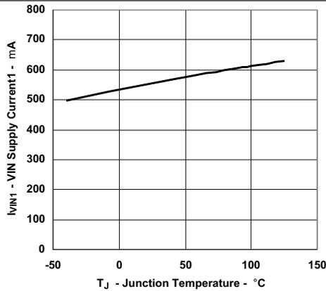
Figure 1. VIN Supply Current1 vs Junction Temperature
