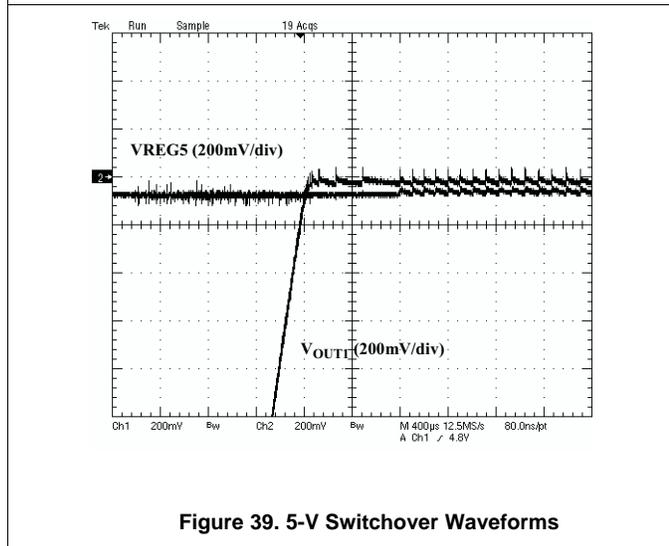
Figure 39. 5-V Switchover Waveforms
