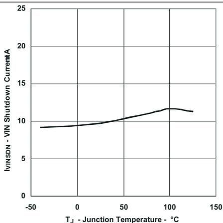
Figure 7. VIN Shutdown Current vs Junction Temperature
