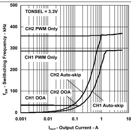
Figure 17. Switching Frequency vs Output Current
