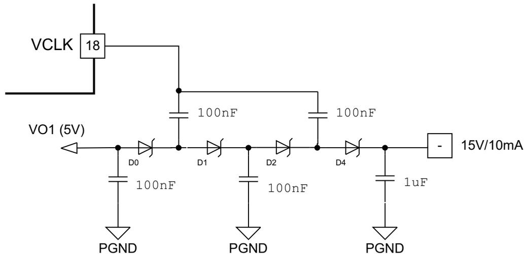
Figure 33. 15-V / 10-mA Charge Pump Configuration
