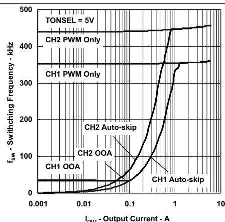
Figure 18. Switching Frequency vs Output Current
