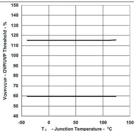
Figure 19. OVP/UVP Threshold Voltage vs Junction Temperature
