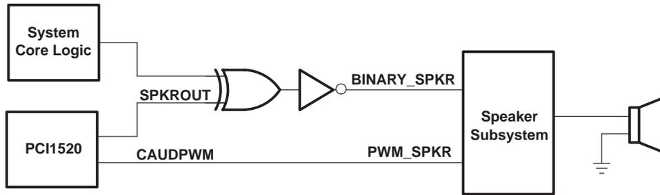
Figure 3-6. Sample Application of SPKROUT and CAUDPWM
