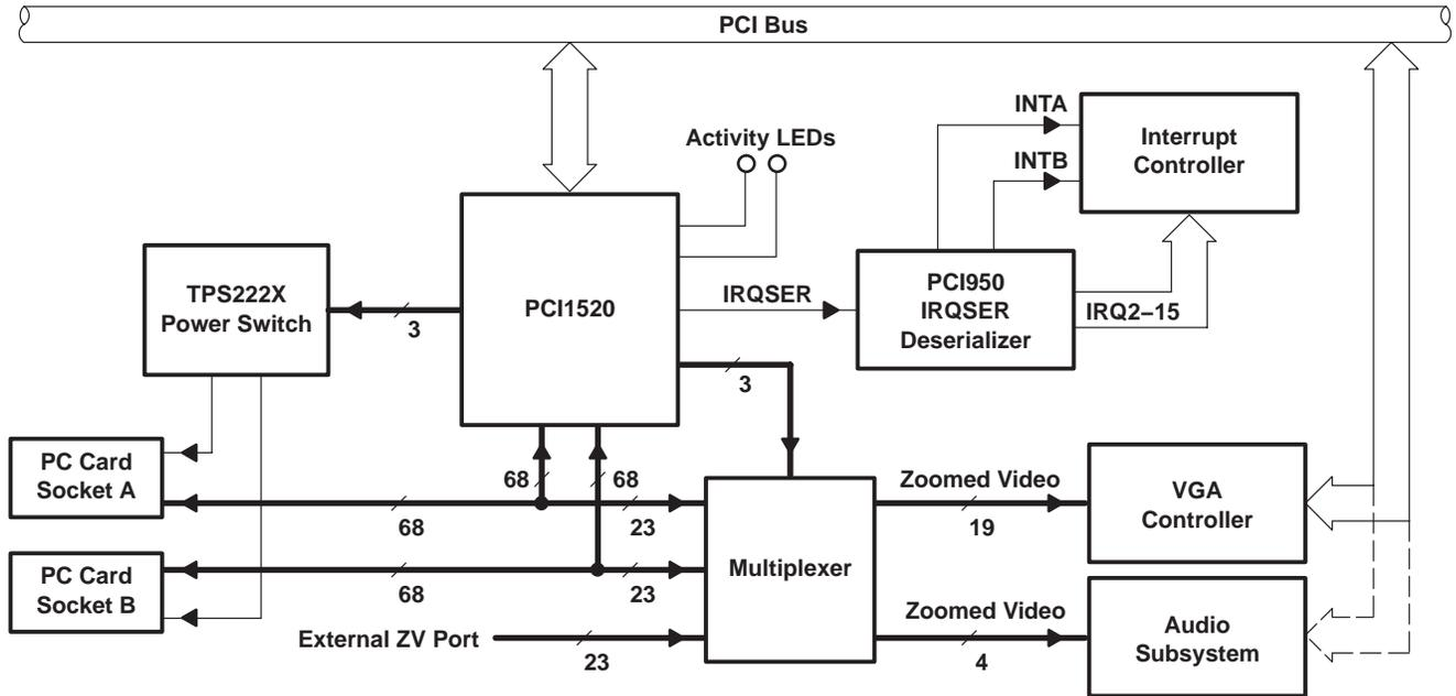
NOTE: The PC Card interface is 68 terminals for CardBus and 16-bit PC Cards. In zoomed video mode 23 terminals are used for routing the zoomed video signals to the VGA controller and audio subsystem.
