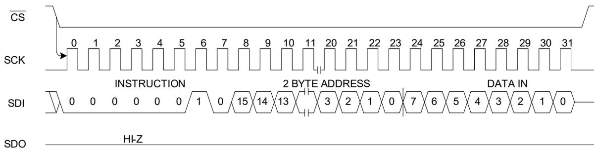
The Adesto RM25C64DS is capable of a 32-byte write operation.
