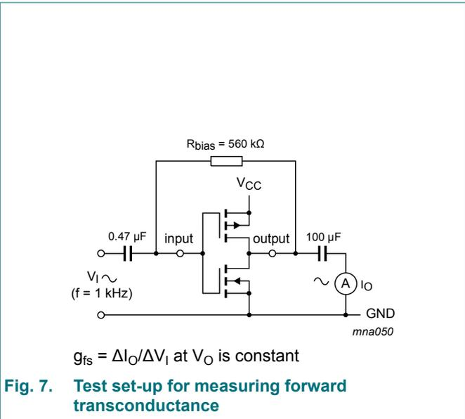
Fig. 7. Test set-up for measuring forward transconductance
