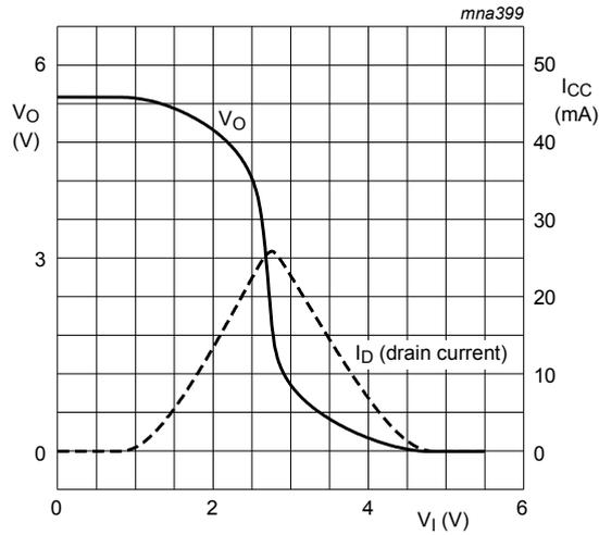
c.  $V_{CC} = 5.5\text{ V}; I_O = 0\text{ A}$
