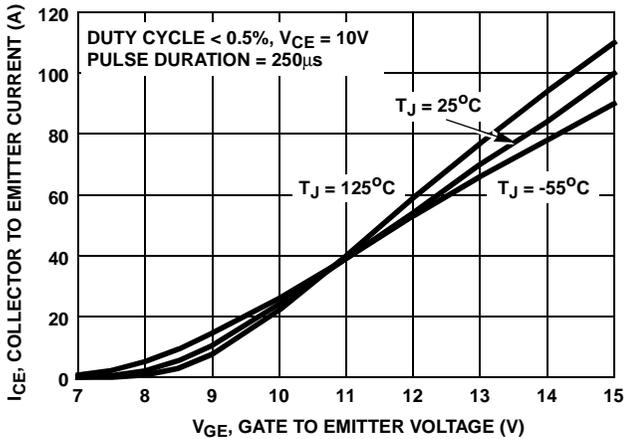
FIGURE 13. TRANSFER CHARACTERISTIC
