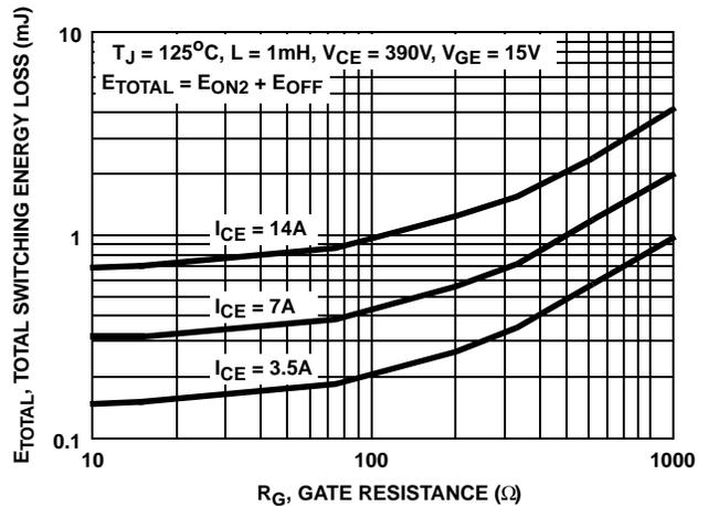
FIGURE 16. TOTAL SWITCHING LOSS vs GATE RESISTANCE
