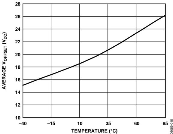
Figure 11. X (Y) Offset Drift vs. Temperature
