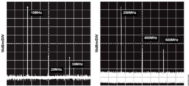
Figure 10. Harmonic Distortion at 10 MHz and 200 MHz;
