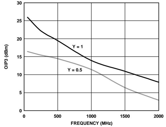
Figure 12. OIP3 vs. Frequency
