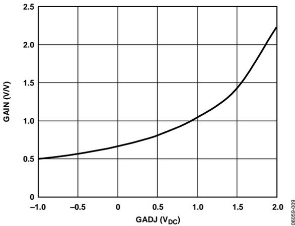
Figure 5. Gain vs. GADJ ( $X = Y = 1$ )
